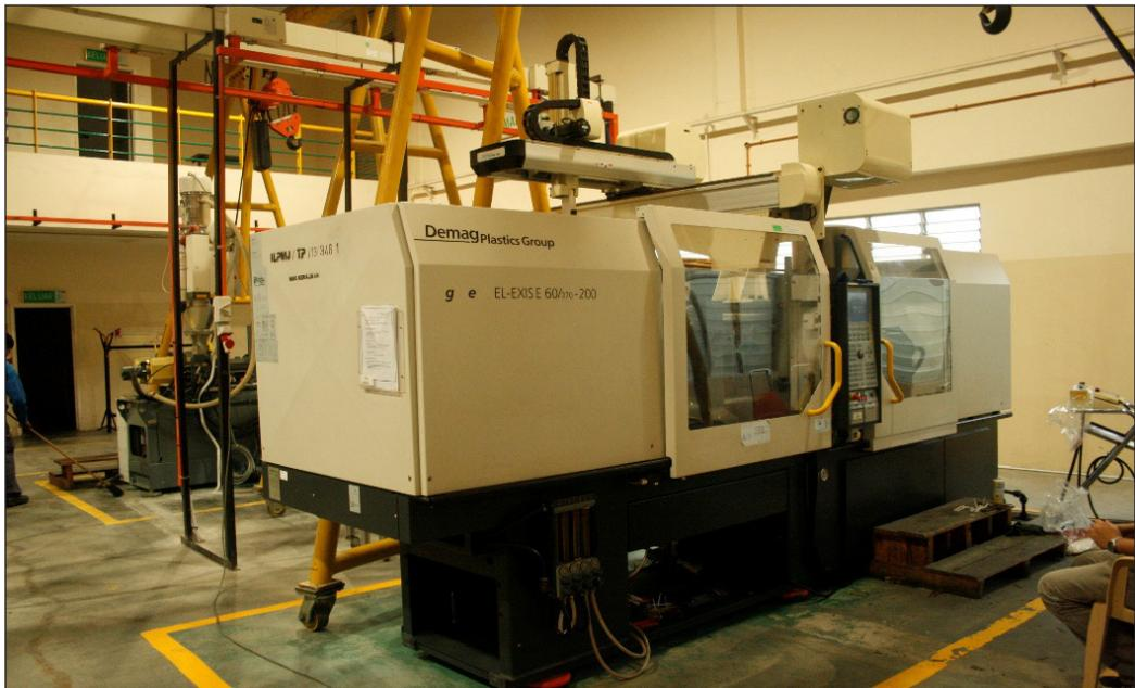
Figure 3. Injection moulding machine Demag EL-EXISE 60/370
