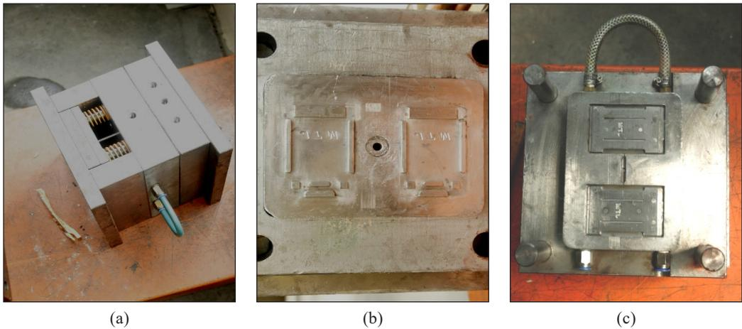
Figure 2. (a) NTP mould set; (b) Female mould of NTP; and (c) Male mould of NTP
