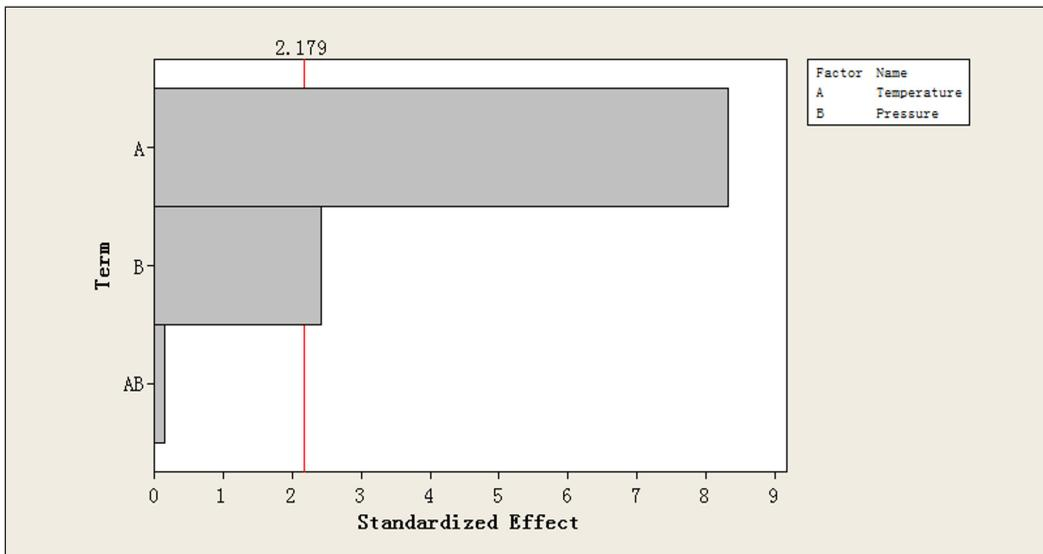
Figure 5. Pareto chart plot of NTP (response is weight, alpha= 0.05)
