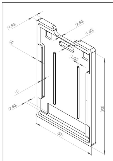
Figure 1. Drawing and measurement of NTP (unit in mm)
